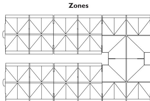
Note: 2 to 3 ft. maximum for straight burners. Longer burners (zones or linear) must use a cross module after every 2 foot straight section due to high temperatures
